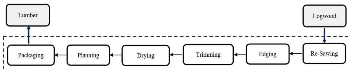
Fig. 3. Key steps of sawmilling process.
