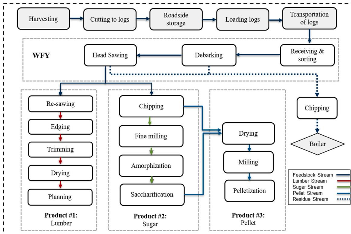
Fig. 2. Schematic representation of key downstream process for the bio-products.
