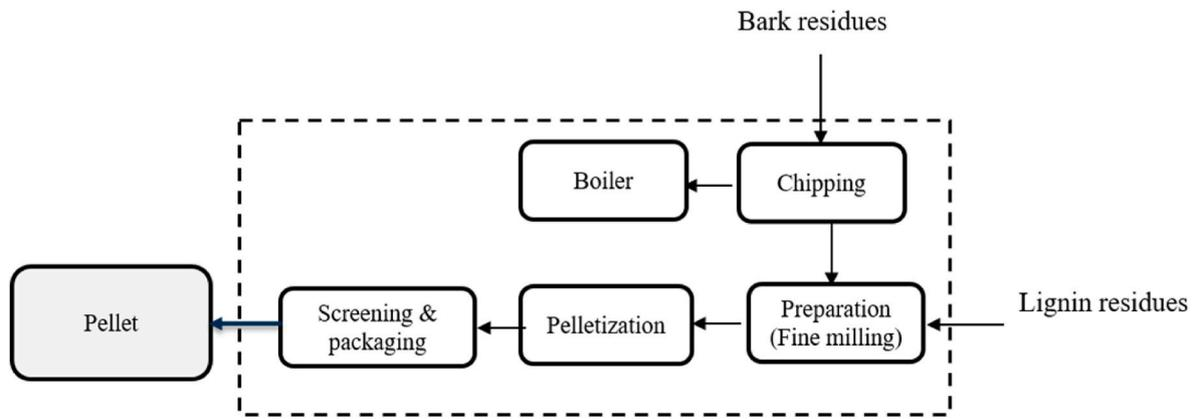
Fig. 5. Key steps of pellet production process.
