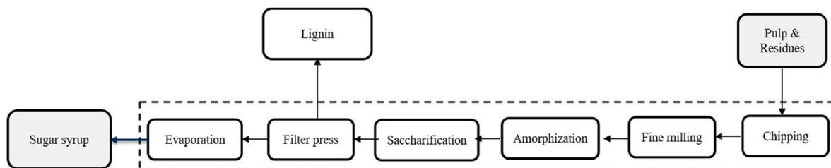
Fig. 4. Key steps of sugar production process.
