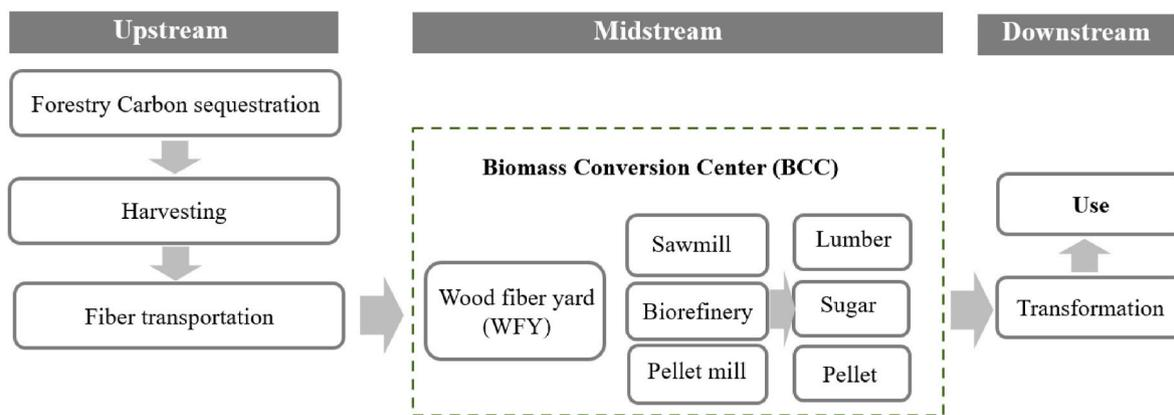
Fig. 1. Cradle-to-Gate stages contributing to cost and GHG inventories of wood based products.
